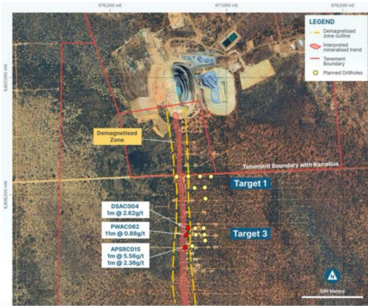
Map of the interpreted mineralised trend, planned drilling and historical intercepts. Pic: SMX
